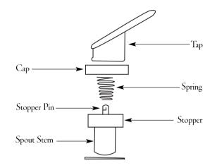
The spout may be disassembled for cleaning as follows:
